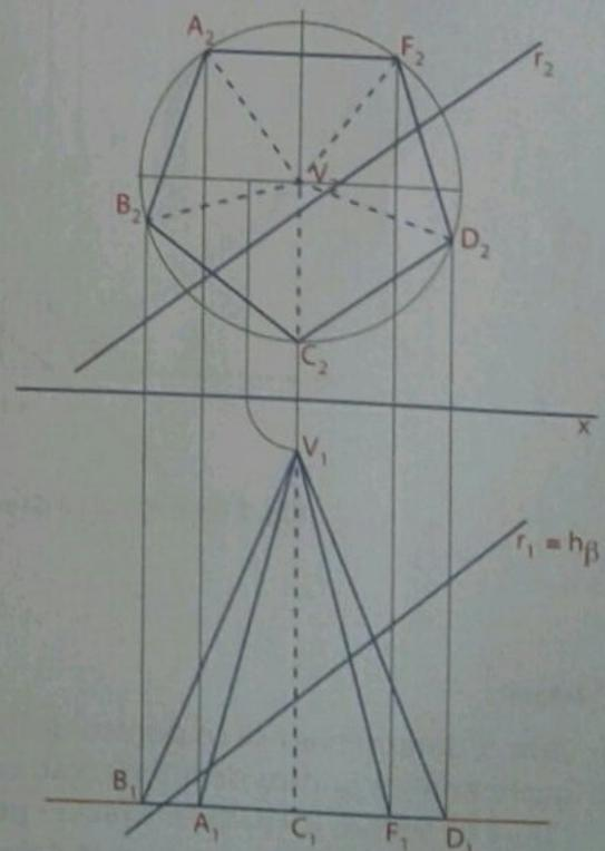
Fig. 6 Conter a recta no plano auxiliar.
